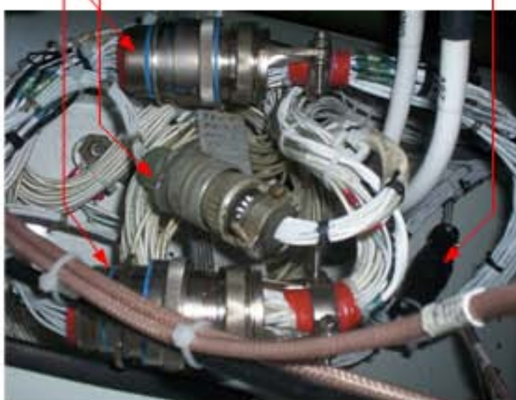
J10 Avionics Disconnect Plug P10 J9 Instrument Panel Main Disconnect P9 J110 Instrument Panel Secondary Disconnect P110 Instrument Panel Keylines Disconnect J25/P25 Left Hand Footwell
